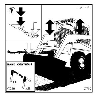
push on the toe of the bucket pedal to dump the bucket. When necessary raise the lift arms to empty the bucket.
